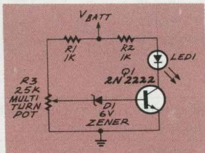
**FIG. 1—WHEN CHARGING NI-CD's, this circuit will monitor the battery voltage and provide you with a signal when a certain, presettable voltage has been reached.**
